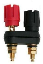
This type of connector is designed to accept flexible or solid conductors. The conductor is inserted into the hole in the post and clamped with the insulated nut. Even if the hole for the cable has a diameter of 4mm or greater and could possibly accept a 4mm banana plug, the connector is acceptable.
